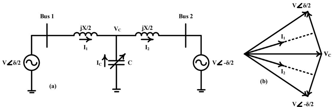
**Fig. 4: Simple model (a) and phase diagram (b) of transmission system with shunt compensation**
