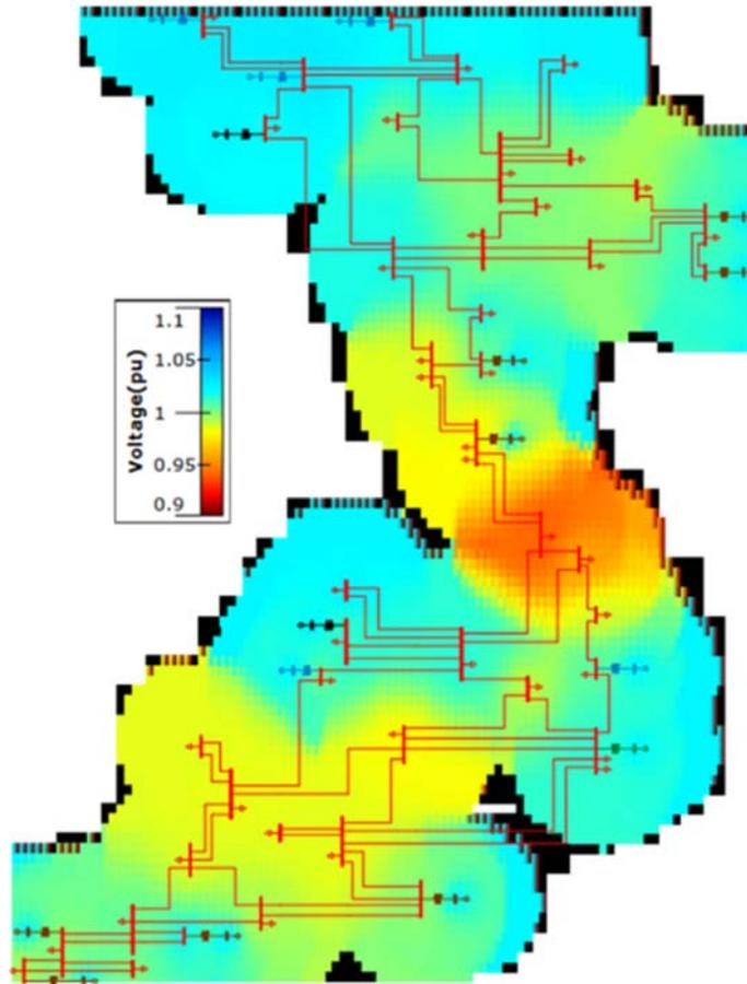
**Fig. 7: Contour-diagram of Vietnam's 500 kV power system at normal operation mode**
