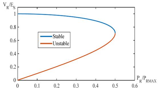
**Fig. 2: The voltage and power characteristics of the simple radial system (Kundur, 1994)**
