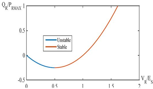
**Fig. 3:  $V_R$ - $Q_R$  characteristics of the system with different  $P_R/P_{MAX}$  ratio (Kundur, 1994)**
