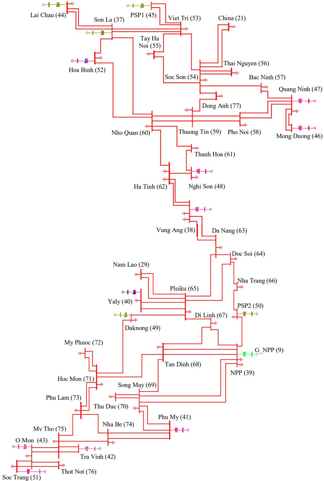
**Fig. 6: Vietnam's 500 kV power system in period 2011 – 2020 with view 2030**
