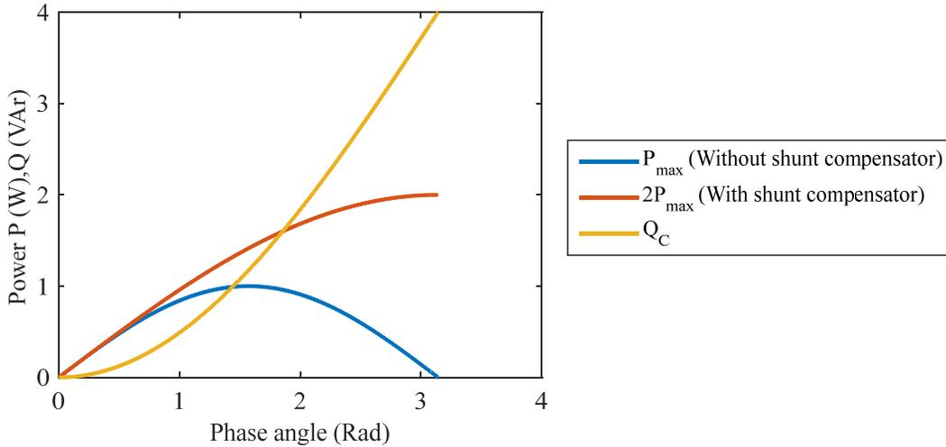
**Fig. 5: The relationship between power and angle of a simple transmission system with shunt compensation**
