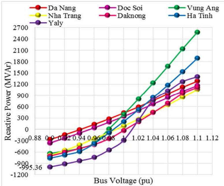
**Fig. 9: Q-V curves of buses with value of reactive power margin lower than 1000 MVar at base case**
