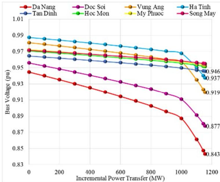
Fig. 12: P-V analysis of buses at single branch contingency between NPP bus and Tan Dinh bus
