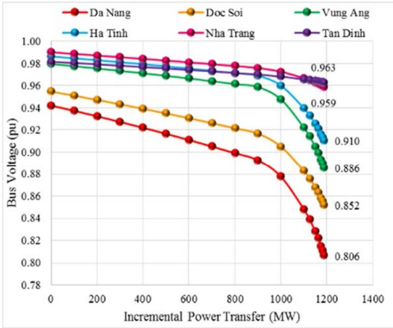
**Fig. 8: P-V characteristics of buses at base case mode**
