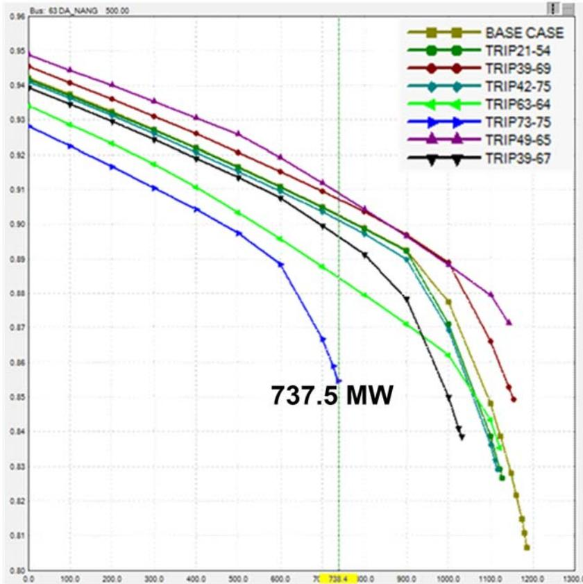
Fig. 10: P-V curves of Da Nang bus at base case and branch contingencies
