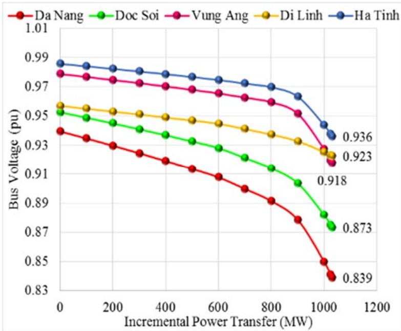
Fig. 11: P-V curves of low-voltage buses at branch contingency between NPP bus and Di Linh bus
