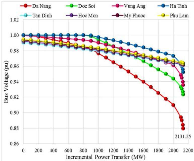
Fig. 13: P-V curves of buses at base case mode with STATCOMs
